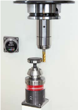
Fig. 1: Thanks to its patented shark360 measuring mechanism, the 3D tool setting probe TC64-20 from Blum enables a high-precision radius measurement to be taken in CNC machining centres. The measurement is taken when the tool rotates backwards.
