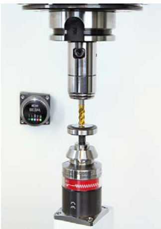
Fig. 2: The universal tool setting probe can also be used for measuring the tool length and for tool breakage detection.
