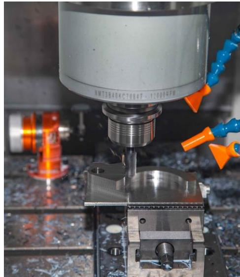
A finish machined selector fork can be produced every cycle thanks to the WNT ZSG vices and MNG Zero Point base plates, while Trochoidal milling techniques using WNT's CCR-UNI milling cutters is reducing that cycle time.
