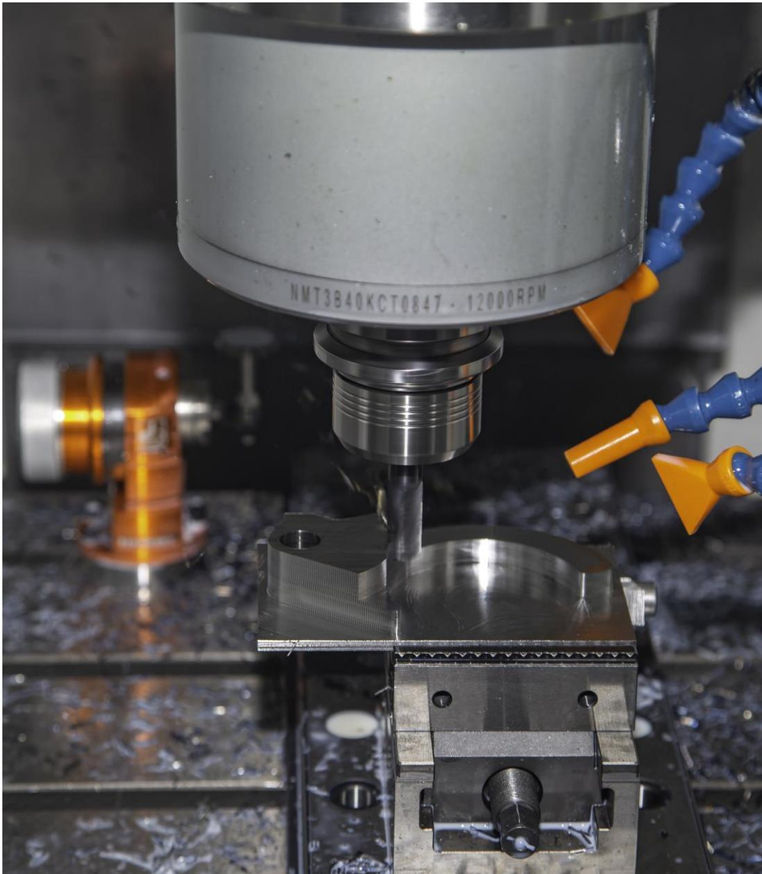
Gripping for the 1<sup>st</sup> operation, which involves relatively high volumes of material to be removed is done using the 80 mm wide ZSG4 vice with serrated jaws, the gripping force for this operation is 65 Nm, the machining of the reverse face of the fork is undertaken in a 125 mm wide ZSG vice, with aluminium jaws, which are
