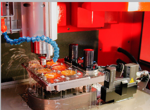
Watch plates in 6-fold clamping
