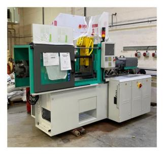
These consist of both Arburg and Engel machinery, the two leading suppliers of Plastic Injection Moulding machines.
