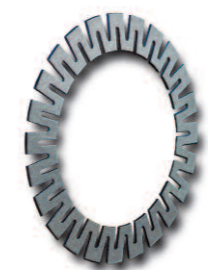
Star Spring Washers as ball bearing compensating discs for taking up free movement in bearings
