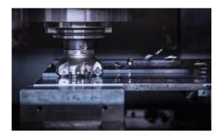
Extending the system size to 12 mm enables more indexable inserts to be attached to the tool holders. This has markedly increased tool lives and chip removal rates.
