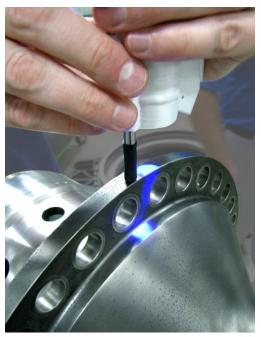
The 4D INSPEC \* instant 3D micro-defect inspection gauge takes the guess work out of 3D micro-measurement, quantifying pits, scratches, nicks, dents, bumps, porosity and other features from 5um-2.5mm deep over a field of view of 8x8mm.
