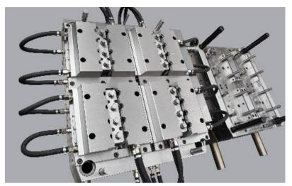
Above: 16 impression tool, running at a 7 second cycle time.
