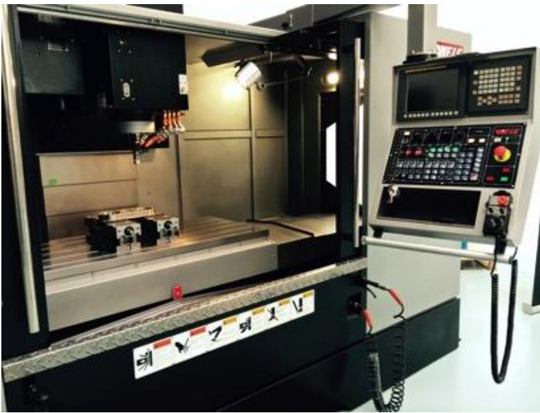
Caption: Wele machining centre with Roemheld machine vices EL 125
