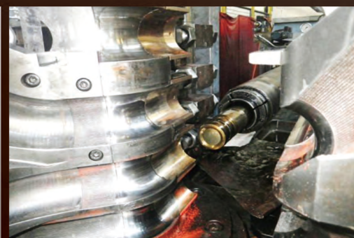
Multi stack dies in AMPCO® 18.23 like mandrel.
