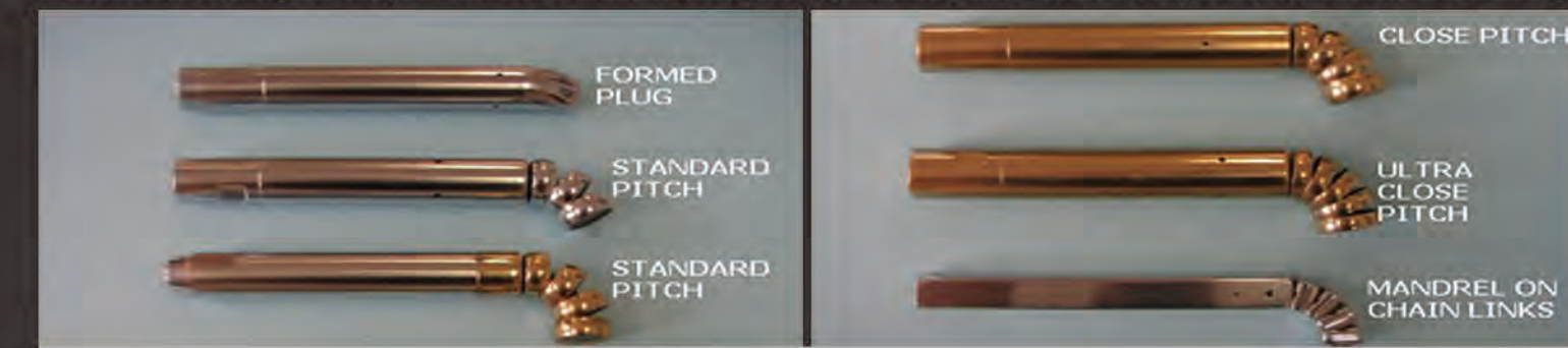
AMPCO® material is useful from simple plug to multiple balls mandrels.
