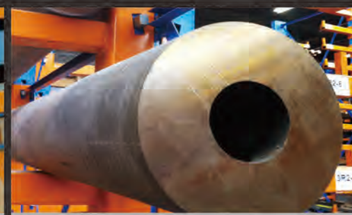
AMPCO® 18 tube for insert wiper dies.
