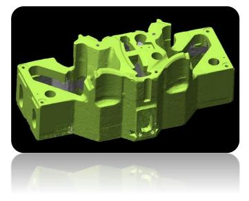
contact-free measurement principle, facilitates rapid measurement of objects which are very difficult to measure using CMM machines.
