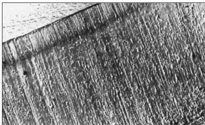
Photo 1. SEM photograph of a D2 punch worn by abrasive wear (work material 1% C-steel at 46 HRC).
