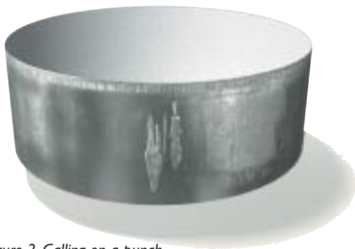
Figure 2. Galling on a punch.
