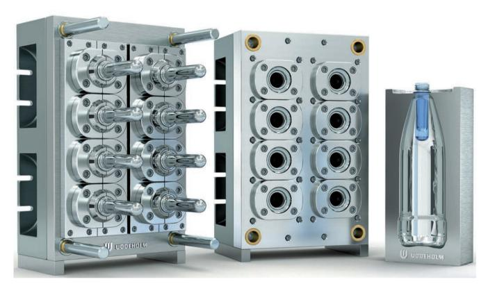
The PET bottles are produced in two steps: first injection moulding of the preforms and then blow moulding of the preforms to the finished bottle. Uddeholm Stavax ESR is a recommended tool steel for production of the preforms.
