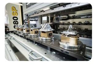
The company's strengths lie in precision machining, steadfast adherence to quality and the ability to tackle complex projects with an extensive machinery arsenal. This comprises of 35 machines, including CNC machining & turning centres and manual cylindrical & surface grinders, as well as a number of cutting-edge automation systems. A double-decker with 33 pallets, feeding a 5-axis machining centre, was the first of its kind in the country.
