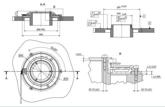
This is just one example of a tailor made encoder kit. For other mechanical, electrical configurations or different interface options please contact us directly: sales@imeasure.co.uk
