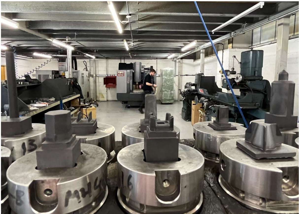
Pictured 1: Electrodes (foreground) with new machining centre (background)
