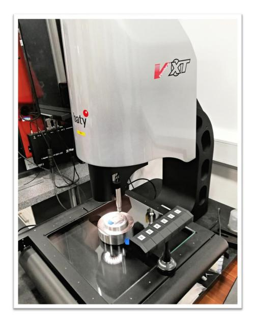
Williams Aerospace Engineering has invested in a Baty Venture XT CNC Vision System to measure critical precision machined components manufactured at their facility in Northam, Southampton. Specialising in 5 axis CNC Turn/Mill Centres, 4 axis Milling, Internal and External Gear and Spline cutting, Internal and External Grinding, Match Grinding and Honing with sizes from 0.062"- 6" Diameter, the business works to tolerances of .002mm (0.00007") with 1 microinch surface finish.
