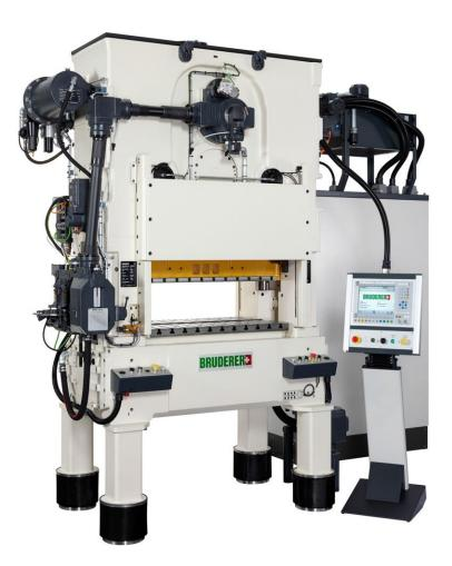
Combining the dynamics of its well-proven BSTA 280 with the performance of a BSTA 510, the new machine boasts a stroke speed of 1600 per minute and an impressive tool loading area of 1100 mm.
