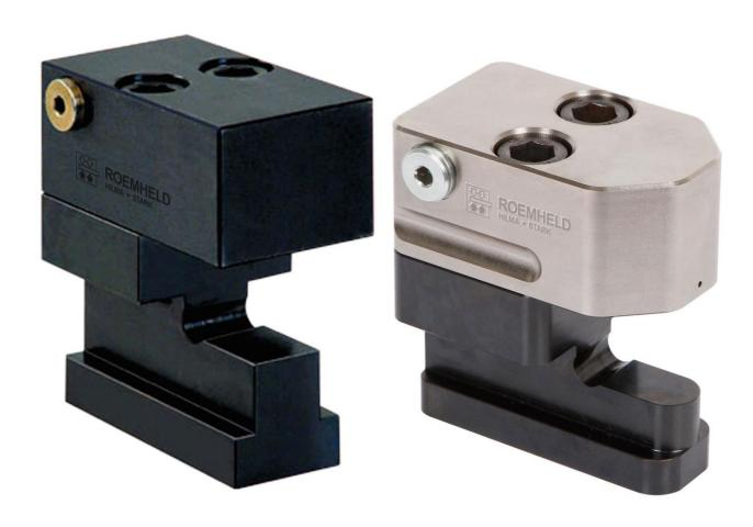
The compact sliding clamp consists of a clamping block and a T-slot adapter which is used to manually position the clamp in the T-slots on the press bed or ram. Various versions are available for the DIN widths of 14, 18, 22 and 28 mm. When used on other systems, the clamping blocks can also be mounted directly without the adapter, for example onto fixed spacer bars.
