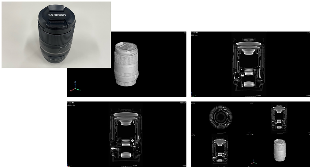
CT image of an interchangeable lens produced by Tamron. Even after completion, the interior can be evaluated without contact.
