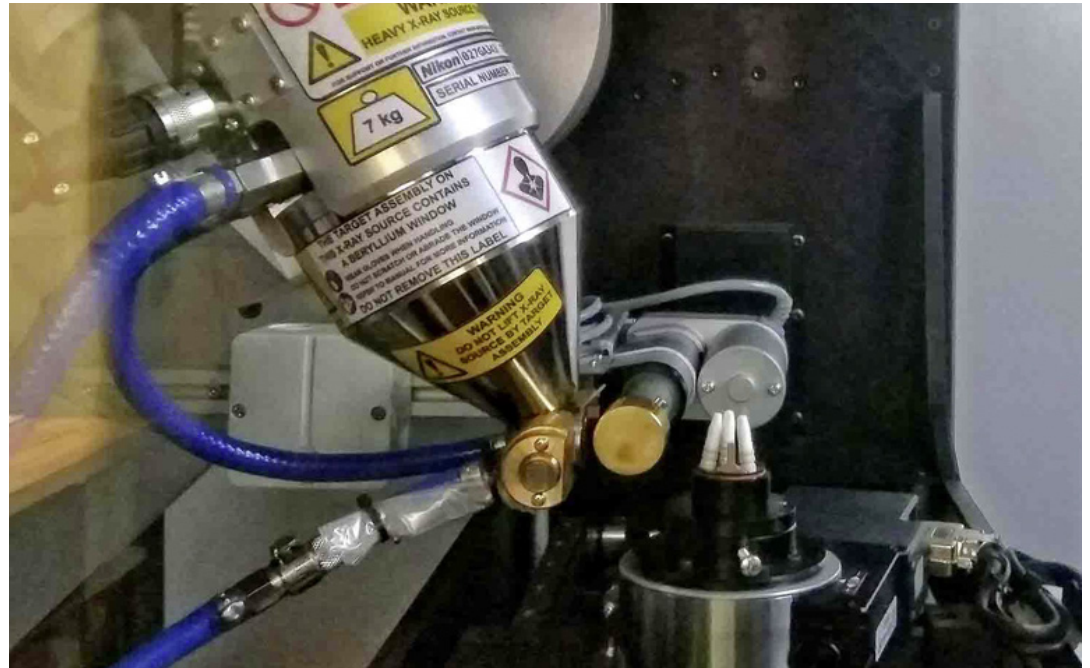
The Nikon Metrology XT H 225 ST X-ray CT system scanning zirconium dioxide implants at Dentalpoint, Zürich.
