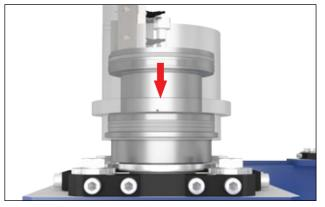
Transfer of hanging frames with CyTab-Scope: in case of reduced ceiling height the transfer can be executed without Z stroke. The frame is fed in Y(X) direction. There is a gap between frame and clamping unit which enables an even lining. Then the unit moves out and clamps the frame sided flange. With that the same accuracy is achieved that is guaranteed by the standard CyTab unit.
