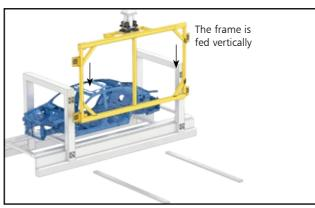
Here also the complete function "gripping • centering • locking" takes place automatically in a single reproducible process. Because of the positive locking the interface is mechanically very stable.
