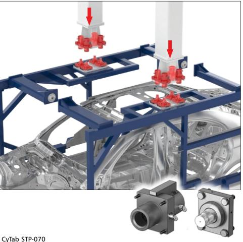
For the frame transfer with vertical axes, we offer the unit STP-070. The high rigidity of the system enables a compact arrangement of the clamping units regarding the required safety in case of an abrupt emergency stop of the machine.
