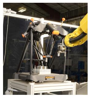
A FANUC robot loads the Equator in the automated cell
