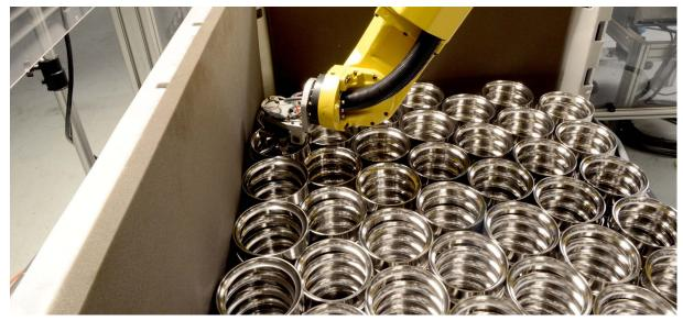
An automated FANUC robot boxes and palletises parts
