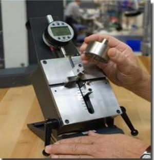
Fig. 2 and 3: Dial Indicators are basically mechanical amplifiers. Digital indicator 1087 R (right)
