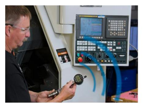
These days, checking parts at a gauging station with a hand tool or a dedicated fixture gauge connected to a computer via a cable for data collection is the norm. Today's hand tools and digital indicators have data output built in and collecting data is easy and very cost effective. It is also inexpensive, fast and reliable providing a great solution for many process or quality control applications.
