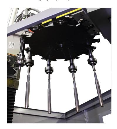
The Single Pass process uses a combination of superabrasive-plated tools, pre-set to exact dimensions, which are passed through the bore, rotating as they complete the honing operation. The number of tools required for any specific task depends on: the amount of material to be removed, the surface finish required and the specified final geometry: roundness, concentricity, bow and/or size.
