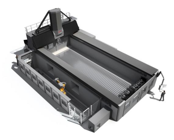
HD characteristics: Excellent machine dynamics mean that the new Droop+Rein FOGS HD (Heavy Duty) can finish items around 20 – 30% faster and more economically than a comparable portal-type milling machine. Images: Starrag
