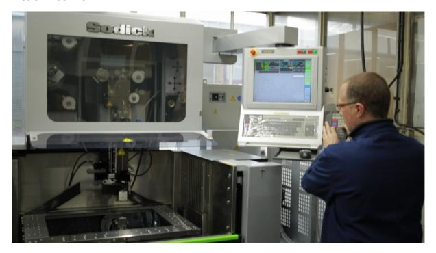
Replacing our older Wire Erosion machine with this machine means we have an increased bed size allowing us to work with bigger parts, higher precision capability with even tighter tolerances, we are able to link 3D models from designer to the on board computer seamlessly and an increase in cutting speeds resulting in a quicker turnaround in parts.
