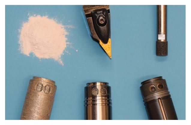
When they arrive, the sintered parts are very rough and granular, so that one of the very first challenges is to decide where the machining datum should be. Also, where conventionally the components would have been machined out of solid bar, the work holding would have been straightforward. With the sintered parts that is not possible, so both machining processes and work holding need to be changed.
