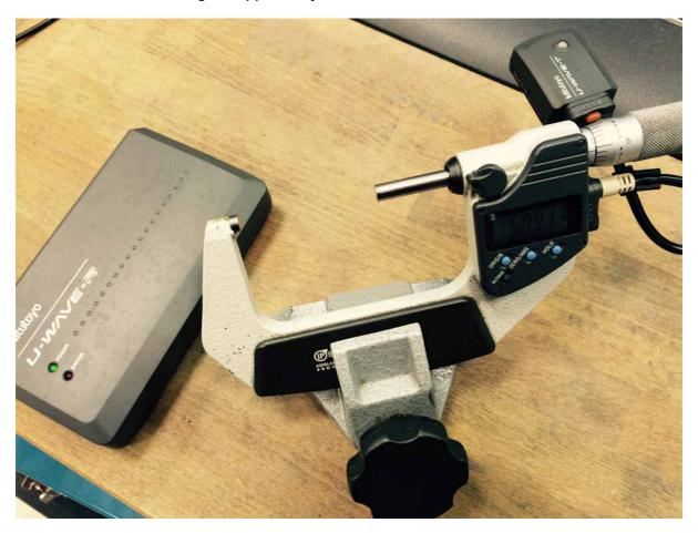
The U-Wave system enables easy wireless data communication from a wide variety of measuring tools, including calipers, micrometers, height gauges, etc. (in fact any tool that provides Digimatic output) direct to a PC. Because the devices are cordless, measurement no longer has to take place near the PC, allowing much greater freedom of layout within and beyond the inspection area.
