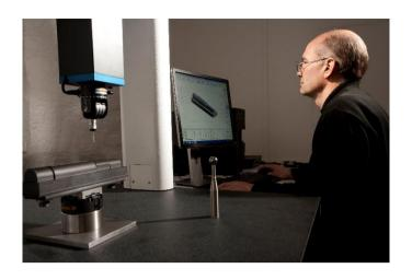
Above: Faulkner Moulds' high end CMM machine measures to an accuracy of 3.5+L/250 $\mu$ m.
