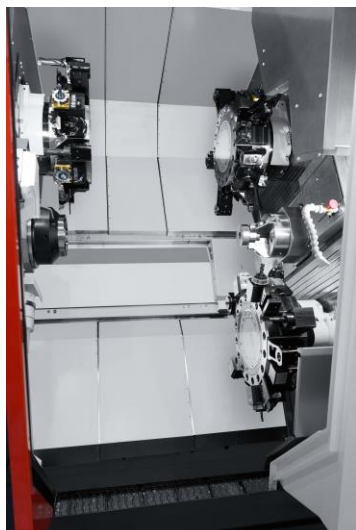
Photo caption 2: The addition of a third turret reduces cycle time by approximately 25%, based on an example component produced with a two-turret configuration.
