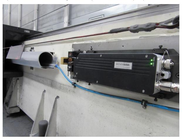
The improved speed allows for the HS20 laser head to be designed into higher velocity applications which are becoming more common in today's manufacturing industries. The aerospace industry is a key market for large machine tools which require long range but highly accurate encoder systems. With throughput being a key consideration in any machine tool purchase, the improved speed of the HS20 ensures that it will continue to be the preferred long range laser encoder of choice.
