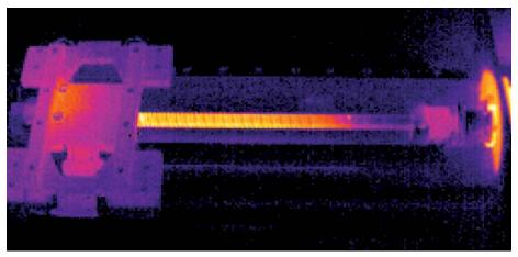
Thermographic image of a recirculating ball screw with increased temperature
