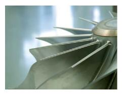
Five-axis machining has long become the standard for the machining of jet engines. High efficiency requirements are driving continuous improvements in the flow characteristics of all jet engine components. The resulting component geometries are very complex and are therefore manufactured exclusively in 5-axis simultaneous milling movements.
