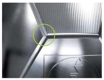
**Closed Loop:** Thanks to the precise linear and angle encoders from HEIDENHAIN, errors in the drive mechanics have no influence on the result of machining. The seams are milled to the correct width, and the intersections all match up exactly.
