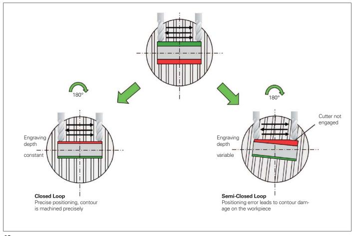
First a workpiece is milled in a **Closed Loop** (see ☑ on the workpiece). Then, a second workpiece is machined on the same machine in a **Semi-Closed Loop** (see ☐ on the workpiece). The difference becomes apparent very soon. While the texts milled in Closed Loop control with precise linear and angle encoders were machined without error on both sides, in the Semi-Closed Loop, machining errors
