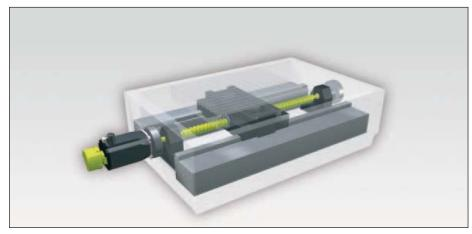
Semi-Closed Loop: Position measurement of a linear axis by a rotary encoder in the feed motor
