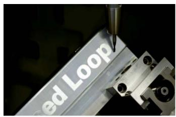
**Closed Loop:** Accuracy-limiting influences from the drive mechanics have no influence on the results of machining. Thanks to the precise angle encoders from HEIDENHAIN, a high contour accuracy and excellent surface definition of the workpiece are achieved.
