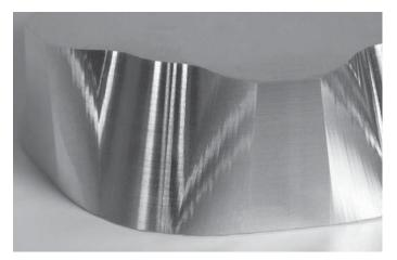
**Semi-Closed Loop:** Polygonal workpiece with surface error.
