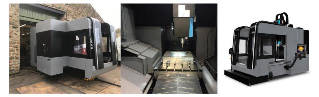
1350 x 950 x 600mm xyz axis capacity. 1500 x 960 table working surface.
