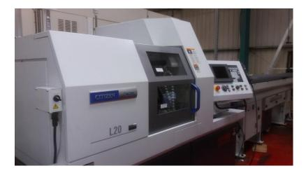
In particular this machine carries an LFV\* (low frequency vibration) function. This is Citizens' latest, unique control technology which oscillates the X & Z servo axes in synchronisation with the spindle. It offers unprecedented levels of chip control and is highly effective for both small diameter drilling and when machining is difficult to cut materials.
