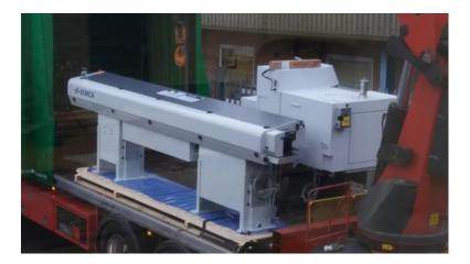
This machine is a Citizen Series 2 L2O-X LFV CNC Sliding Headstock Turning Centre. The L2O has adopted a modular design, but also focuses on operability and working convenience. The high level of basic performance found in features like the position adjustable operation panel that makes it possible to monitor the interior of the cutting room while looking at the operating screen.
