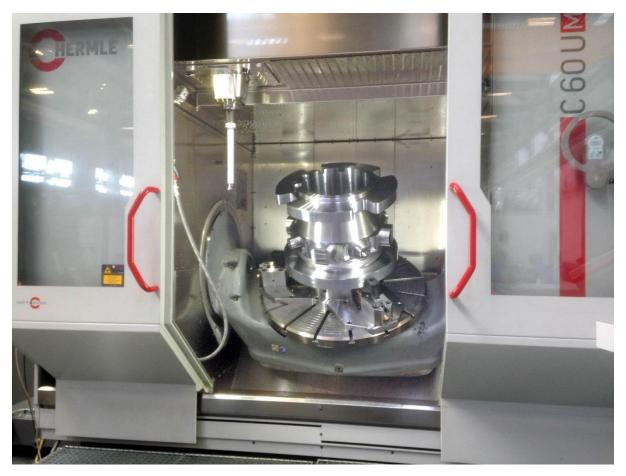
Many features of the machine and control combination were presented, three of which are worthy of special mention. One was 'A-axis Turning', which allows the trunnion to be continuously positioned at any angle while the component on the table is rotated for turning using a fixed tool in the spindle. The merits of this simultaneous interpolation to improve cutter access and allow shorter turning tools to be used for more stable machining were readily appreciated by the audience.
