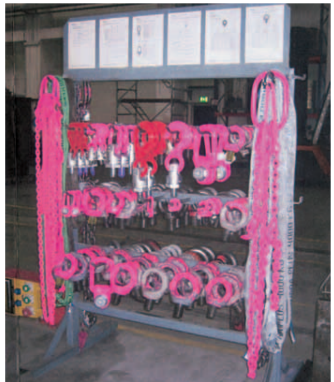
Correct storage of lifting points and sling chains BGR 500.
