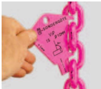
Testing for plastic elongation caused by overload
