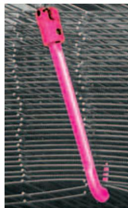
The bevelling on the back of the hook simplifies the horizontal hook insertion between the bales. The clevis connection enables a direct chain connection and the integrated ball bearing swivel prevents the chain from automatically spinning.
