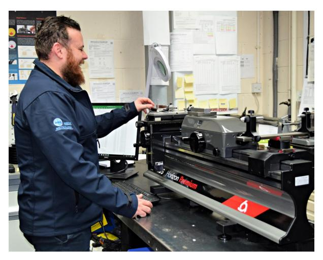
Mech Metrology is now able test screw ring gauges and internal threads in house, a job that would have been previously subcontracted out. The Trimos Horizon Premium has also improved MECH Metrology's output, as well as significantly increasing the efficiency of the calibration process.
