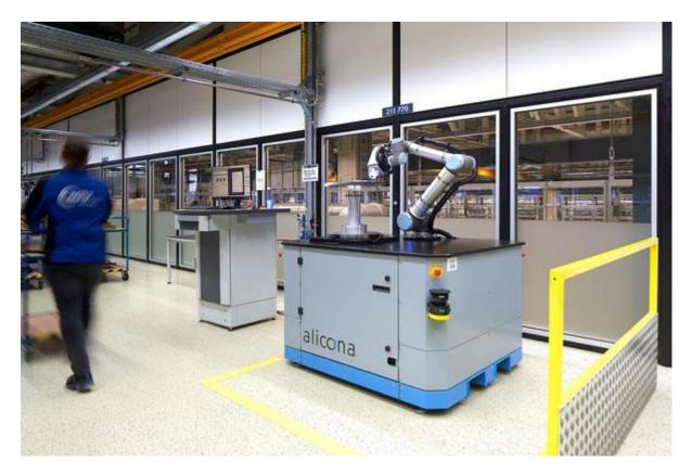
Cobots consist of a collaborative 6-axis robot and a high-resolution optical 3D measuring sensor and are a popular measuring device for production-integrated quality assurance.
