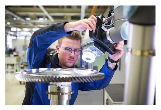
The operation of the Cobots is designed for the use of several operators. Handling, measurement and evaluation by means of programmed test routines are easy to handle, as MTU confirms.
