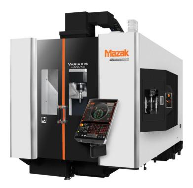
The VARIAXIS j-500/5X delivers high accuracy and productivity from a wide A-axis spectrum of rotation (+30° to -120°). Outstanding accuracy is guaranteed by its high rigidity structure, which utilises linear roller guides on all linear axes and roller gear cam on both rotary axes.
