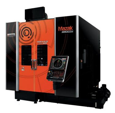
The Wire-Arc AM torch is mounted on the machine's headstock to deposit material layer-by-layer and grow near-net-shape 3D forms. The system quickly deposits material due to the use of wire instead of metal powder.
