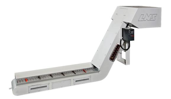
The LNS system has a built-in scraper bar attached to the hinge belt that continuously runs along the bottom surface of the conveyor frame throughout the machining cycle to gather even the smallest chips. The swarf is then lifted onto the top of the conveyor as the belt rotates and is able to exit in the same manner as the larger swarf.
