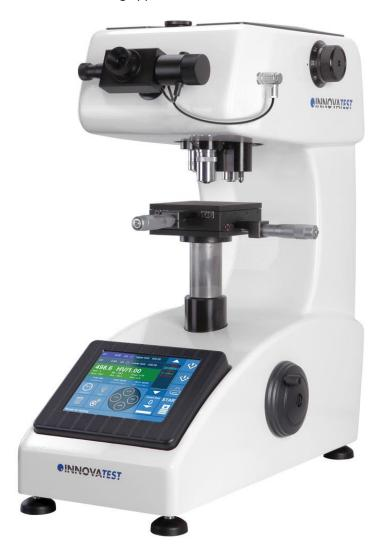
The NOVA 130 features a three position turret which includes one indenter position as well as a 10x and 40x objective. The NOVA 240 is well equipped for more demanding applications, featuring a four position turret including one indenter position, as well as 5x, 10x and 40x objectives.
