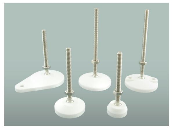
The nickel-plated or stainless steel nuts resist corrosion even under high pressure or chemical washdown conditions, while the smooth white polymer bases are free from nooks and crannies where dirt and debris can accumulate. The bases are also infused with an anti-microbial agent that is effective against the growth of bacteria.
