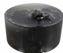
Sample impregnated with KEPT using KemVac
