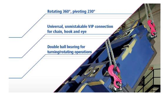
The demand for loads to be turned, swiveled and rotated safely during the handling process of a project has certainly increased over the years. Loads can easily be damaged and lifting systems can be considerably overloaded. Mould and die manufacturers are prime examples of this, when moulds or dies must be flipped the lifting points they use need to swivel and pivot at the same time.
