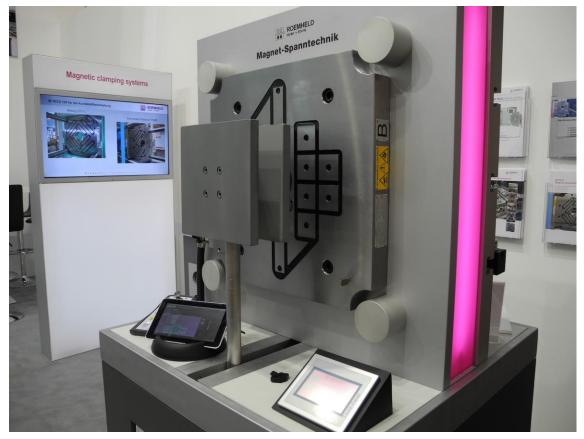
The new Roemheld controller satisfies the highest safety requirements of performance levels "d" and "e" for mould monitoring, power supply, magnetisation and emergency stop. All safety signals and error messages are displayed on the control panel, or can optionally be simultaneously transmitted via RS or Profibus interfaces to the press controller.
